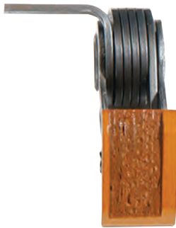
A cam tensioner from an engine that used the manufacturer's conventional oil.
