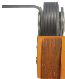
A cam tensioner from an engine that used the manufacturer's synthetic oil.
