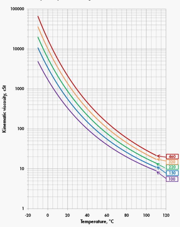
Viscosity - Temperature Diagram for Shell Morlina S3 BA
